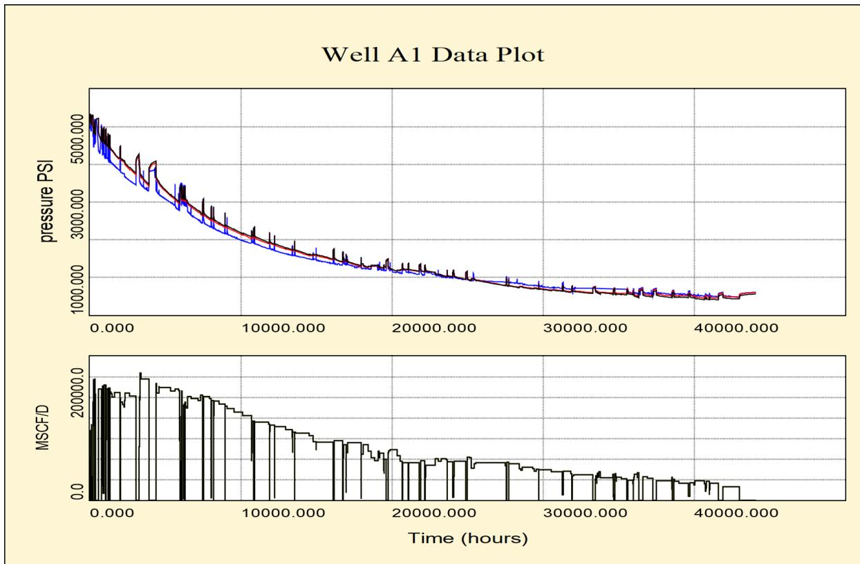
**Fig. 9. Simulated pressure behavior based on the four-region model vs. the pressure prediction based on the reconstructed pressure response.**
