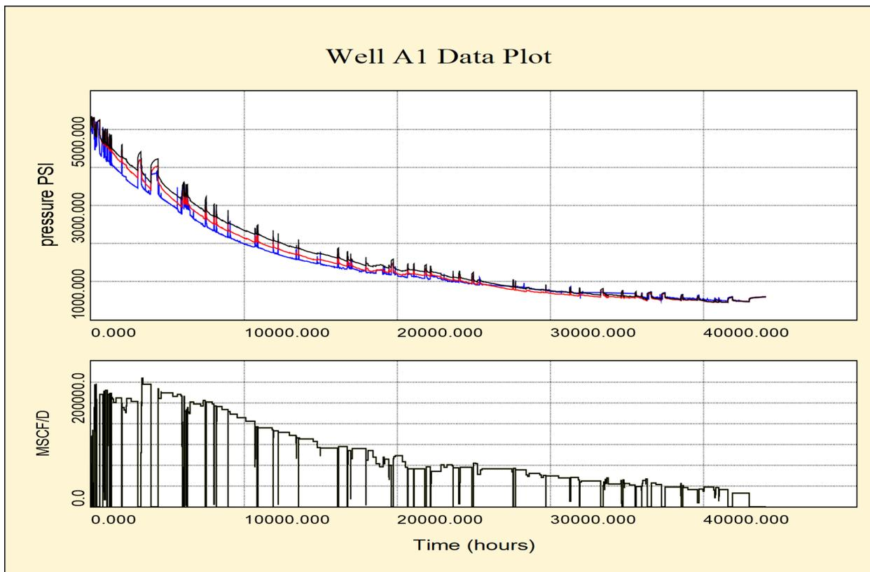
**Fig. 5. Simulated pressure behavior vs. the pressure prediction based on the reconstructed pressure response.**
