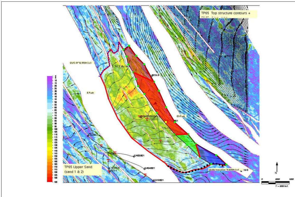
**Fig. 6. Four-region reservoir model. The three red solid lines in the plot split the reservoir area into four polygon regions.**
