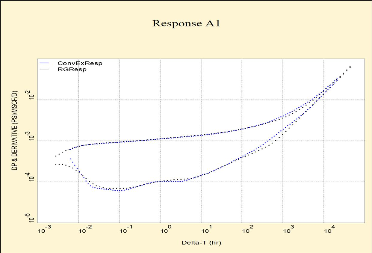
**Fig. 4. Comparison of reconstructed and simulated unit-rate drawdown responses.**
