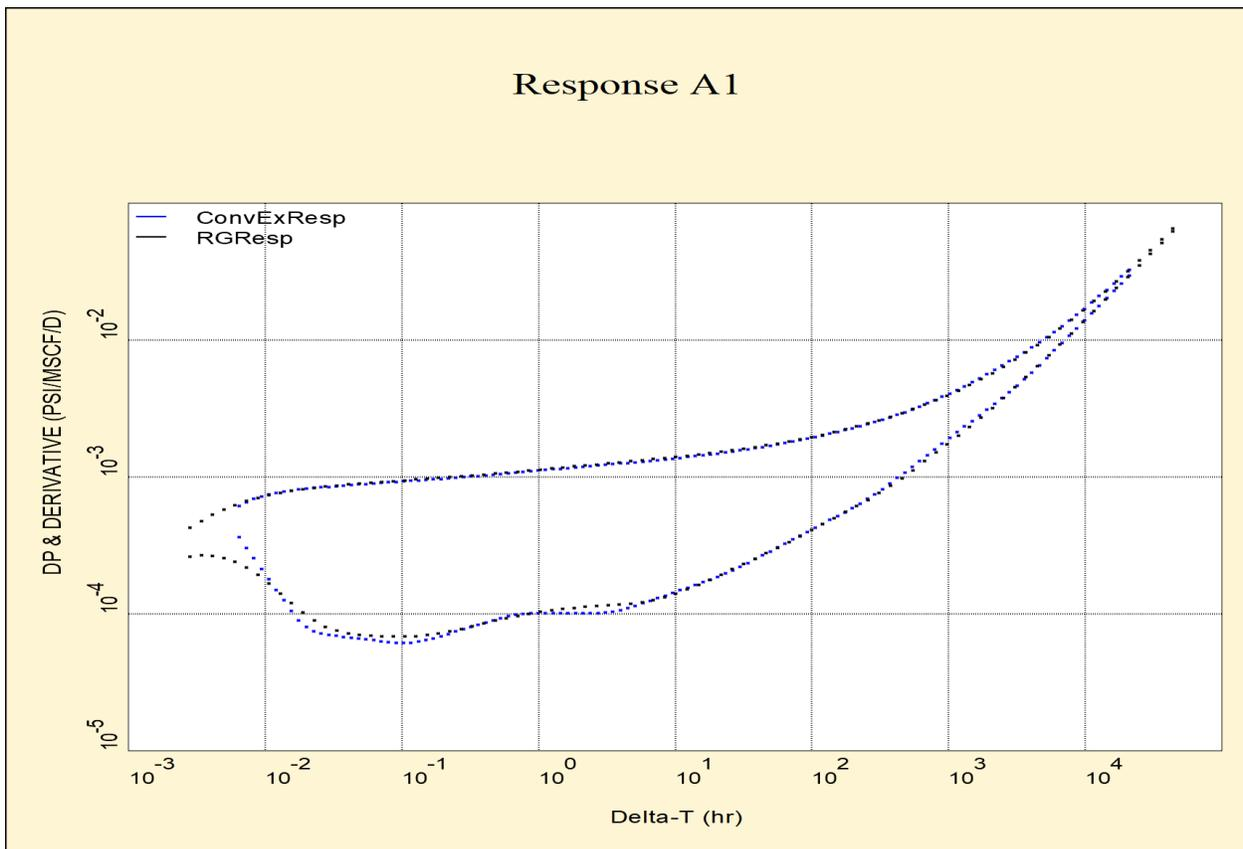
**Fig. 8. Comparison of reconstructed and simulated unit-rate drawdown responses using four-region model.**
